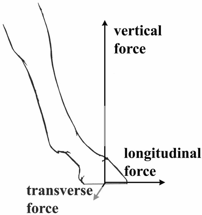
Figure 1: Vertical, longitudinal, and transverse components of the ground reaction forces.
