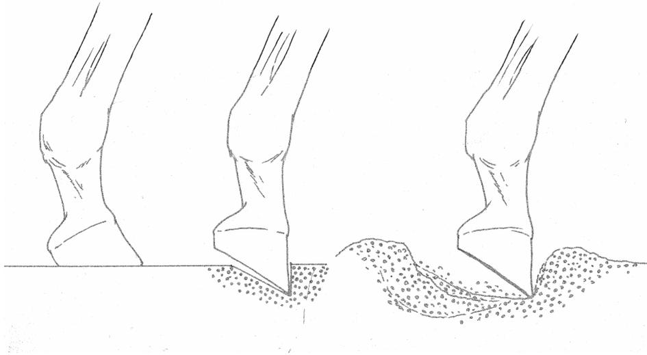
Figure 1: Effect of shear resistance of the surface. Surfaces with high shear resistance do not allow the toe to penetrate (left). Surfaces with intermediate shear resistance allow the toe to penetrate but offer sufficient resistance during push off (center). Surfaces with low shear resistance give way as the hoof pushes off (right).
